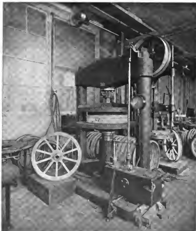
Fig. 35—Hydraulic press which forces the rims on to the woodwork after the rim has been expanded by heating to about 600 degrees C. A pressure of 25 tons may be exerted
